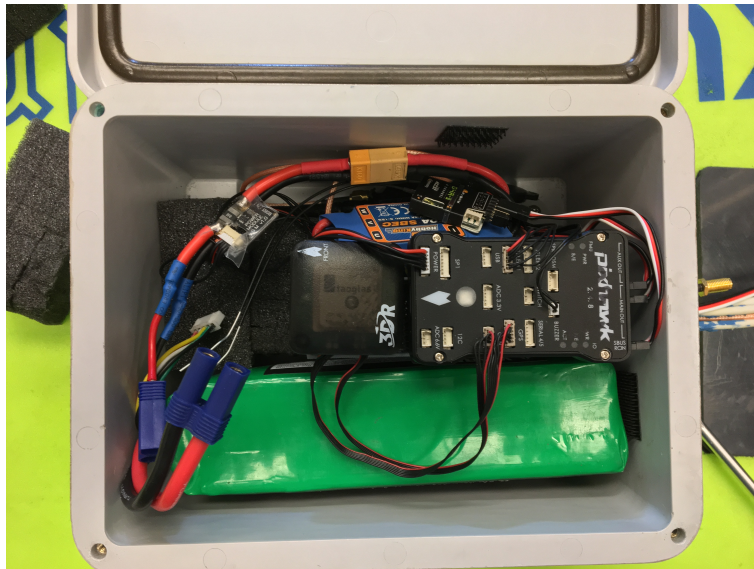
Figure 9: The devices use compasses to guide the board, so they must be oriented correctly. The front of the board is on the left side of the image.
