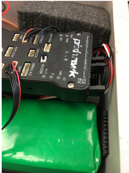
Figure 8: Note the orientation of all of the cables. Ensure everything is plugged in to the correct port with the correct polarity.
