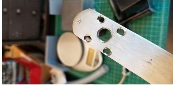
Figure 2: You might need to widen the preexisting hole if the motor shaft diameter is too large.
