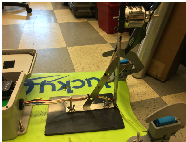
Figure 3: Ensure that the bracket is mounted with all required hardware to avoid failure.
